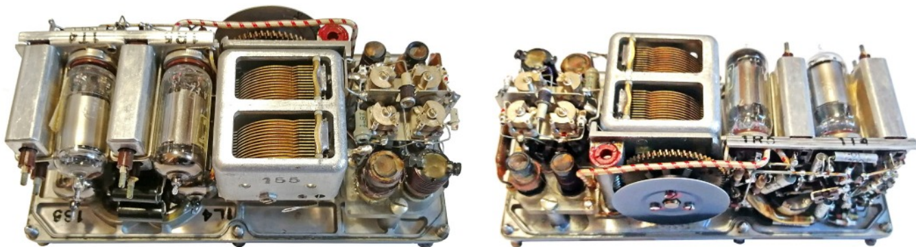
Internal view of the RR.24A receiver revealing the use of Philips IF transformers and tuning capacitor.
